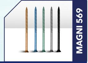
Magni 569 is a hex-chrome-free duplex coating that combines a plated zinc and non-hex chromate substrate with a durable Magni chrome-free organic topcoat. Engineered for use on fasteners, deck screws and other building hardware, Magni 569 provides superior product performance in fewer layers than comparable finishes.
