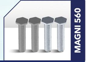
Magni 560 is a chrome-free duplex coating that combines electroplated zinc and hex-chrome-free passivated substrate with an aluminum-rich organic topcoat. A coating that can be engineered to specific coefficient-of-friction needs, Magni 560 is offered with exempt solvents and typically applied to fasteners, including nuts, bolts and other hardware. Magni 560 can be applied via dip-spin or spray application methods.
