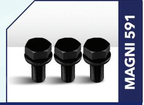
Magni 591 is a duplex fastener coating that combines an inorganic zinc-rich basecoat with an organic topcoat. Engineered for use on fasteners, including nuts, bolts and other hardware, Magni 591 contains integrated friction modifiers and eliminates the need for sealers or post-coating lubricants; this ensures repeatable torque/tension characteristics in assembly. Magni 591 is applied via dip-spin, dip-drain or spray application methods.
