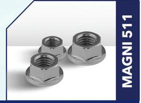
Magni 511 is a chrome-free duplex corrosion protection coating that combines an inorganic zinc-rich basecoat with an organic topcoat and is engineered for use on fasteners, including nuts, bolts and other hardware. Formulated with integrated friction modifiers to eliminate the need for sealers or post-coating lubricants, Magni 511 ensures repeatable torque/tension characteristics in assembly and is applied via dip-spin, dip-drain or spray application methods.
