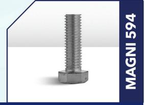
Magni 594 is a chrome-free duplex fastener coating that combines an inorganic zinc-rich basecoat with an aluminum-rich, friction-modified topcoat. Engineered for use on fasteners, including nuts, bolts, screws and other hardware, Magni 594 offers fewer processing steps, resulting in improved quality and reduced costs. Magni 594 can be applied via dip-spin or spray application methods.
